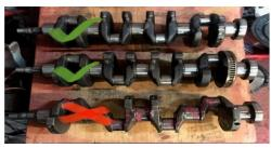
Only the crankshafts ticked green permitted twin web NO single web cranks. Internal engine parts must be as x16xel y16xe z16xeand to the sizes given
