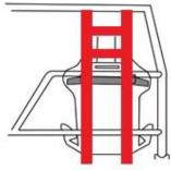
Seat should be in front of b/pillar hoop [if not] a twin drag car type bars must be fitted off roll cage hoop to either the back bars or the roll cage or if it goes to the floor it must be sat on 23cm square plate 3mm (min.) thick. These two bars must be connected around the head height with at least two connecting bars. This new section must not be constructed in a way that a drivers helmet can make contact with it. Material od and thickness as rest of roll cage.
