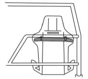
If the seat sits behind the b/pillar hoop a secondary support to the cage must be added. An example of this is shown in the diagrams within this section of the document. If the modification goes to the floor it must be sat on 23cm square plate 3mm (min.) thick.
