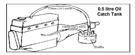
An oil catch tank, with a minimum capacity of 0.5 litres, must be fitted in the engine bay, and must have a minimum of two breather pipes connecting to it, one from the rocker box and one from the crank case. If the catch tank becomes ineffective during racing or practice, the car will be withdrawn from the event.
