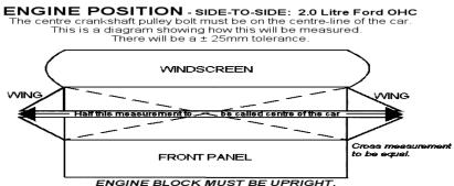
The centre crankshaft pulley bolt must be on the centre-line of the car. There will be a ± 25mm tolerance.
