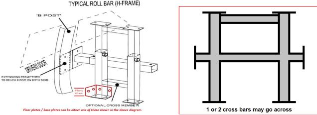
These two diagrams are a guideline to how the frame should be constructed but gusseting or triangulation is accepted.
