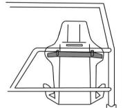
If the seat sits behind the b/pillar hoop a secondary support to the cage must be added. An example of this is shown in the diagrams within this section of the document. If the modification goes to the floor it must be sat on 23cm square plate 3mm (min.) thick.
