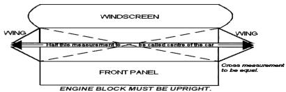
The centre crankshaft pulley bolt must be on the centre-line of the car. There will be a ± 25mm tolerance NB: Both Wings must be the same width (i.e. no offset panels).
