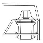
If the seat sits behind the b/pillar hoop a secondary support to the cage must be added. An example of this is shown in the diagrams within this section of the document. If the modification goes to the floor it must be sat on 23cm square plate 3mm (min.) thick.
