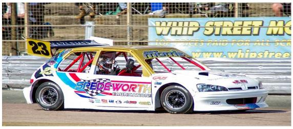
**A.** Any four-seater, front-engined, saloon or hatchback, constructed of steel, the overall length must not exceed 3988mm (157") and the overall width must not exceed 1702mm (67") when ready to race. Consideration will be given to any modern vehicle which falls outside these specified measurements in its original form, but can comply when prepared for racing, as follows:
