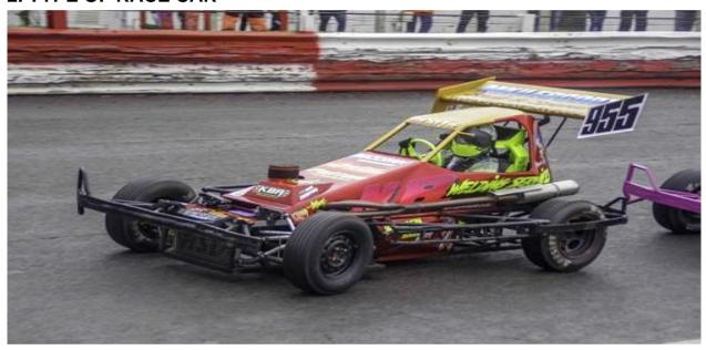
The Race car must be of an open wheeled chassis design, with a front longitudinally mounted engine, driving the rear wheels. The driver's cockpit must be behind the engine, but in front of the rear axle and be central to the main chassis rails.
