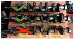
Only the crankshafts ticked green permitted twin web NO single web cranks and must be in the original form.
